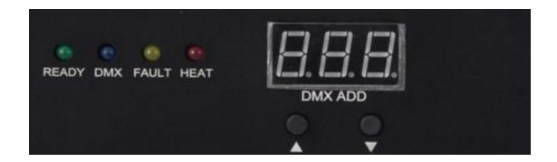
**READY:** Green light Flash indicates that the system is ready for work, and the steady light indicates that the system could work now
